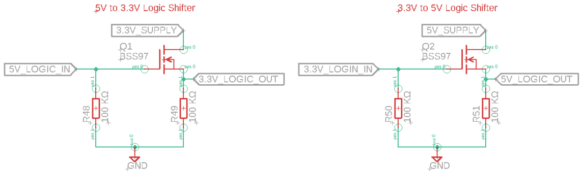
Figure 5.26: Charge Controller Input and Output Level Shifters
